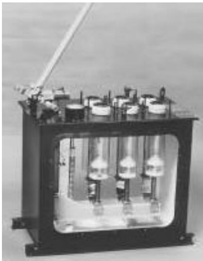
SF6 Puffer action is self-generating using the SF6 contained in the switch tank. Arc extinction occurs at first current zero.
