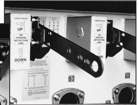
Photos below: Interrupter operating handles for manual single phase (below) or three phase (left) operation and reset. Motor actuators can be added to three phase for remote operation.
