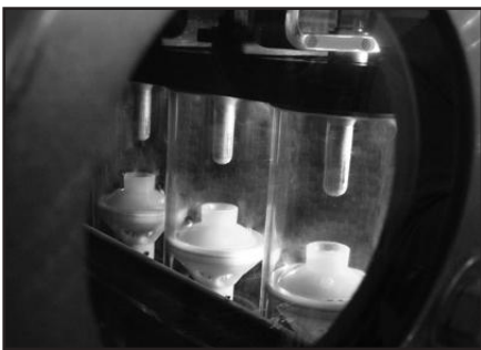
▲ Three phase visible position of contacts.
